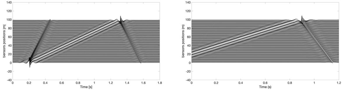
FIGURE 3 – Vertical displacements induced by a moving load, computed using a SEM solver with (Left) homogeneous initial conditions and (Right) heterogeneous initial conditions, at sensors located along a line parallel to and 2 m away from the loading line.
