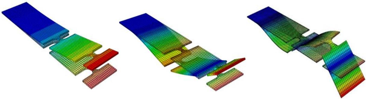
Figure 7 – Simulation of the 3 first flexional modes
