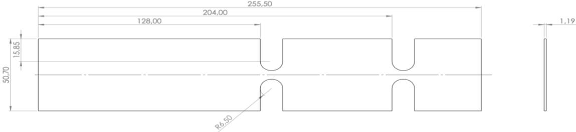
Figure 1 - Specimen geometry
