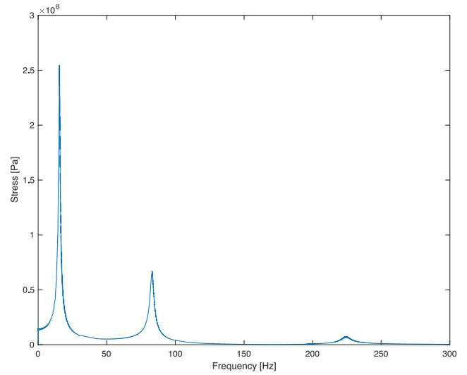
Figure 9 – Simulated max stress-FRF
