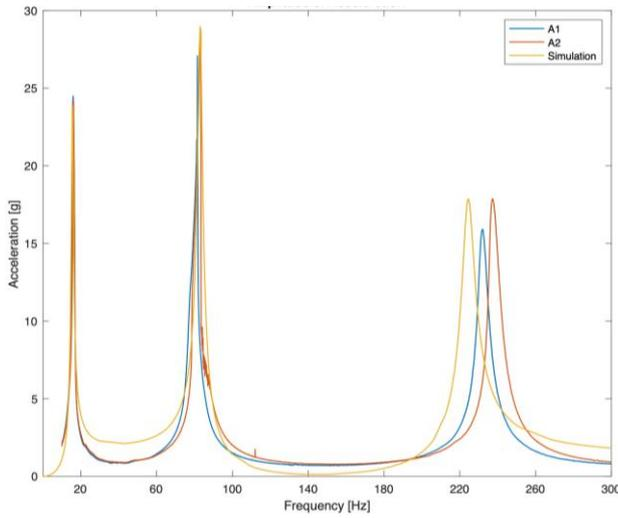
Figure 8 – Experimental and simulated FRF accelerations.
