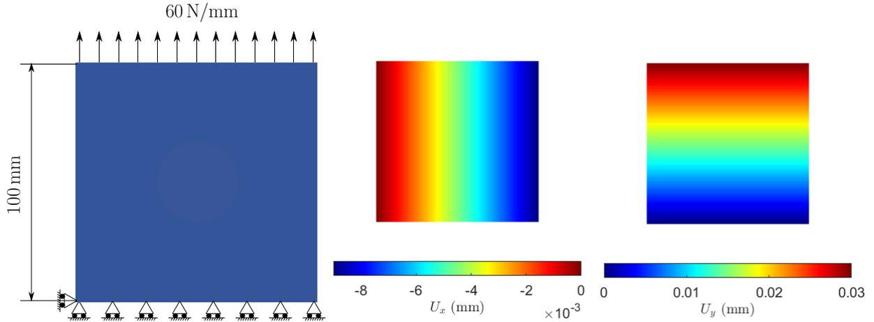
FIGURE 2 – Reference structure and the corresponding displacement fields
