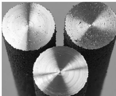
Figure 5: Printed specimens, with different parameter sets. Differences in the pore sizes are clearly visible.
