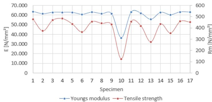
Figure 6: Tensile test results, for the 2x17 specimens, of grid “a” and grid “i”.
