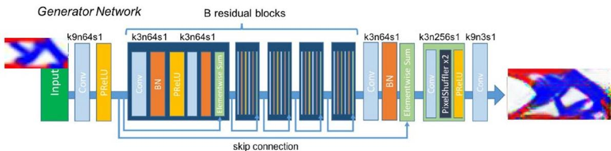
Figure 2 Generator Network Diagram
