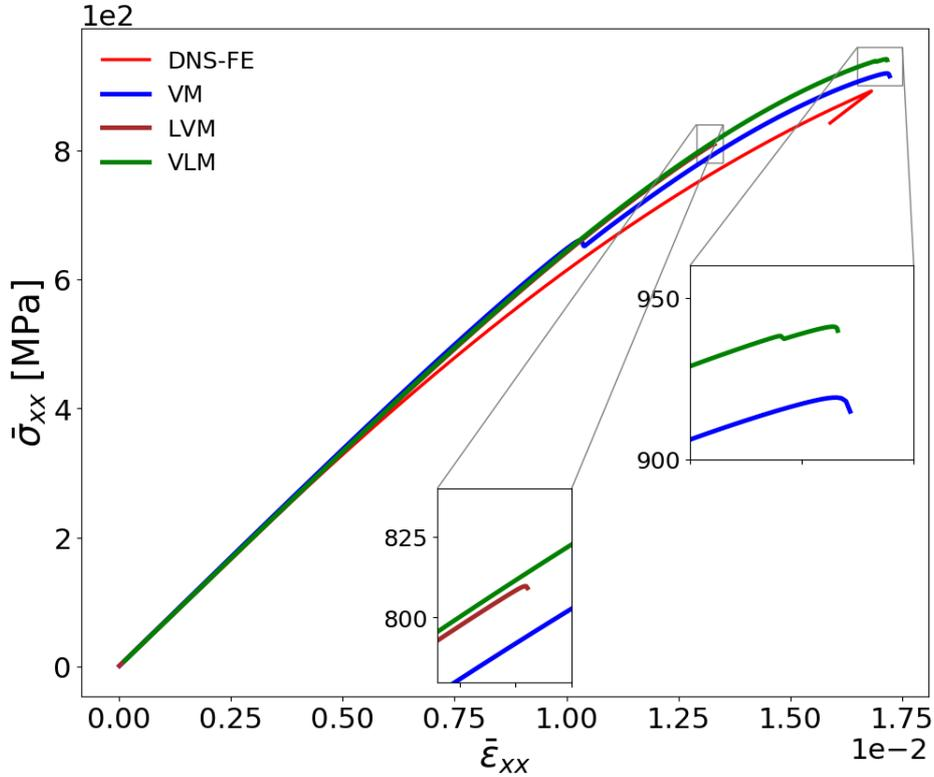
Figure 6: Uniaxial tensile test on the RUC
