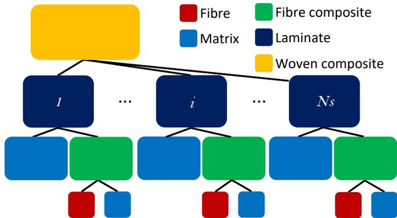
Figure 5: Computational network of the VLM scheme.
